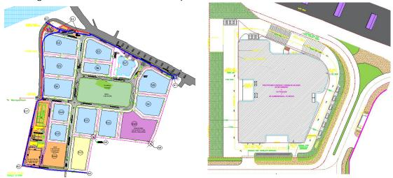
Total built up area of Fintech Tower is around 5.5 lakhs sq.ft. with 2 Basement + 3 Podiums + 9 Floors structure. Basements and podiums are for parking.
